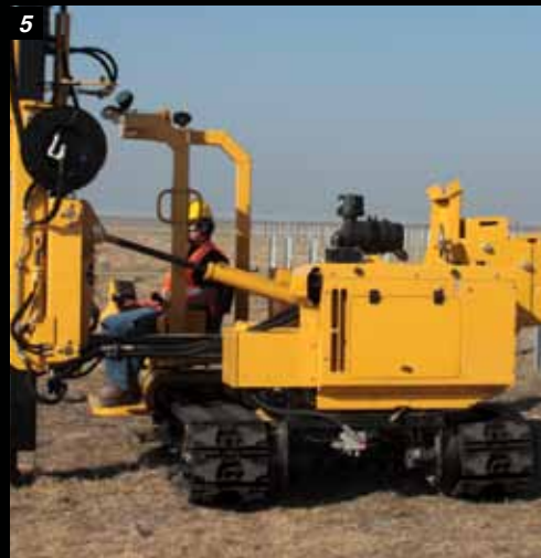
6: Operator options. Operators can choose to be seated or to use an optional wireless remote control, which controls machine functions, including hammer engagement, pile placement and ground drive.
